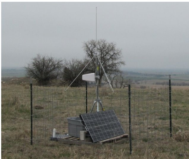
Fig. 4. Portable Lightning Mapping Array (LMA) Station.
